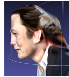
FIGURE 9. A limitation of training on SmartPortraits: the back is never visible in the dataset, leading to poor reconstructions or occluded regions beyond the ears.
